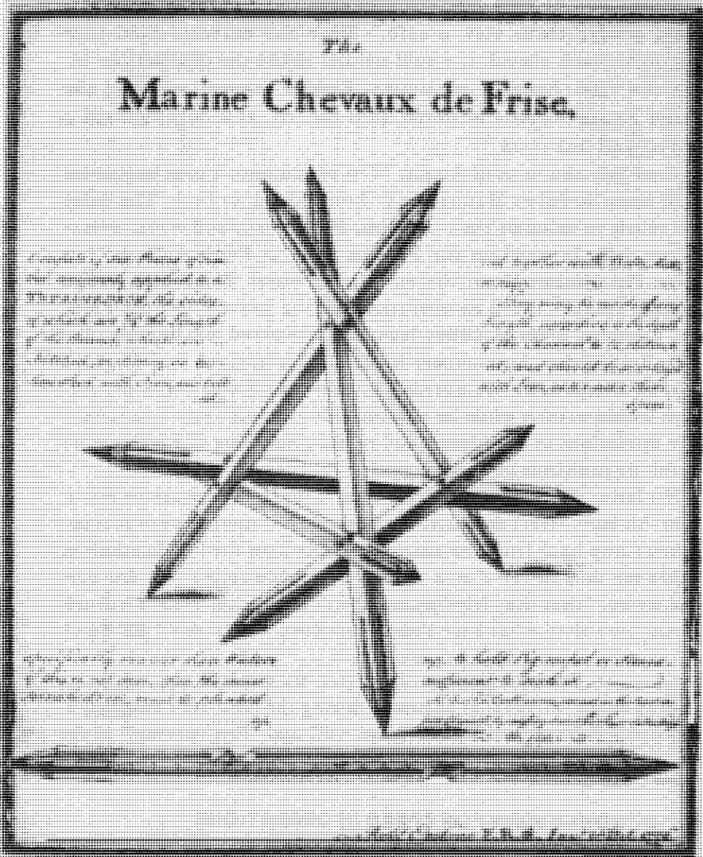
ROBERT ERSKINE'S CHEVAUX-DE-FRISE. Although used for obstructions in the Hudson River between Forts Washington and Lee, Erskine's design was deemed impractical for Philadelphia because of the soft floor of the Delaware River. American Philosophical Society
